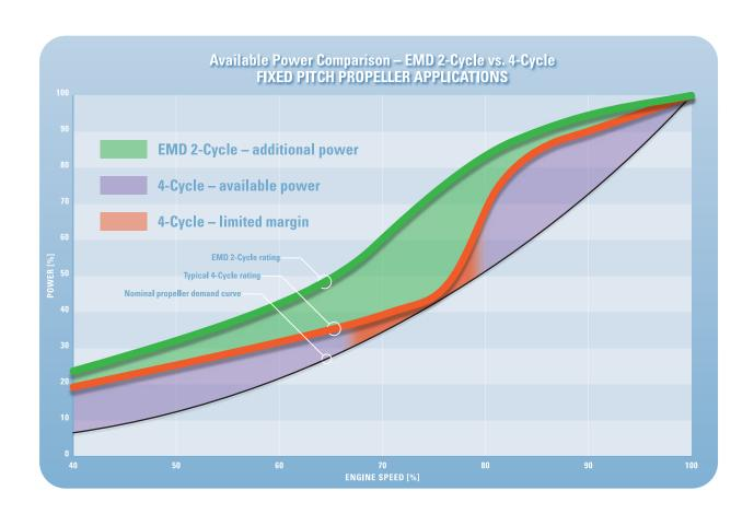
The EMD 2-cycle engine provides a large margin of available power above the demand curve to provide superior acceleration and responsiveness. By comparison, in fixed pitch propeller applications, the available power of a typical 4-cycle engine narrowly meets the propeller demand curve, especially in the middle to upper engine speed range.
